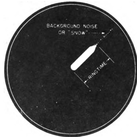
Figure 2-4. Ringtime Indications on Plan Position Indicator, Antenna Stopped
